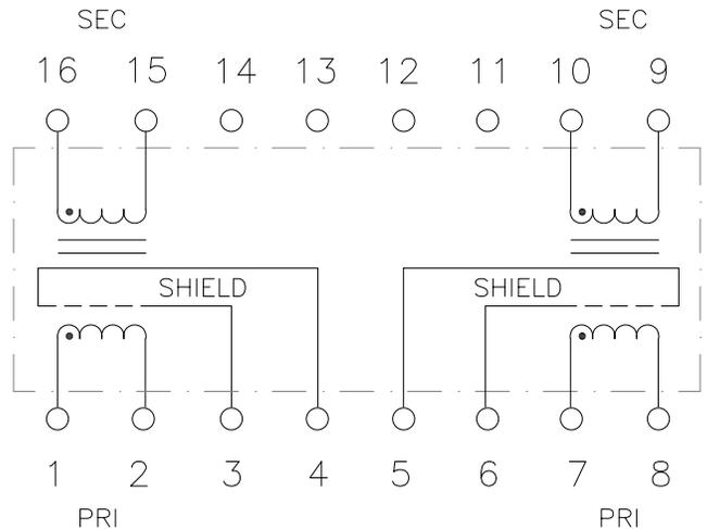
Only one end of the shield can be grounded
